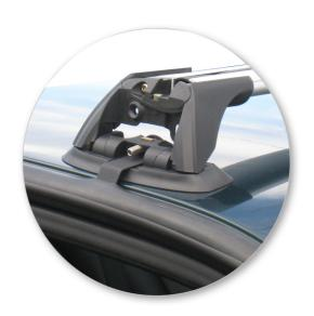
• Refit rubber seal over the clamp.
